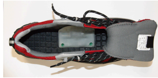
Figure 2. Pressure sensitive insole used in the experiment. The device is shown (a) outside the shoe and (b) inside the shoe. In black, the array of pressure sensors covered by a silicone layer. In white, the housing for the processing and transmission electronics. Picture from [1].
