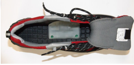
Figure 1. Pressure sensitive insole used in the experiment. In black, the array of pressure sensors covered by a silicone layer. In white, the housing for the electronics. Picture from [5].
