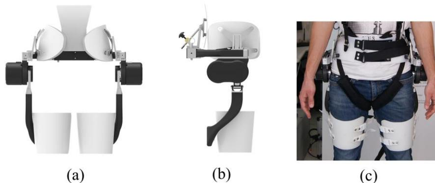
Fig. 1. Overview on APO. a) CAD frontal view. b) CAD lateral view. c) Frontal view of a subject wearing the device.
