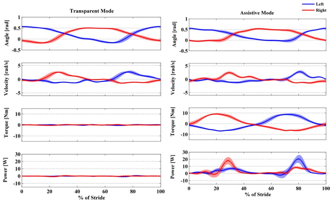
Fig. 2. Walking with the APO under TM and AM. For each gait speed, the following variables for left and right hip joints are averaged over all strides and plotted against the percentage of the stride cycle: hip joint angle, hip joint velocity, SEA torque and power. For each graph the average curve (solid line; blue for left and red for right joint) is shown along with the standard deviation contour.
